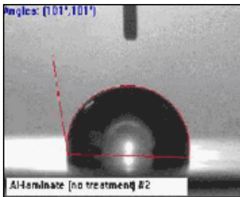
Figure 9A. Contact angle of a water droplet on an untreated surface. [5]
