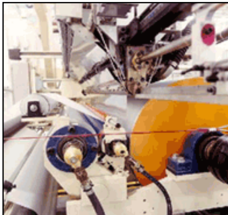
Figure 3 left is the extrusion lamination section of the extrusion coating line at Great Lakes Technologies. Here we can see the spreader roll leading into the nip section, the backup cooling roll, the nip (or pressure roll), the ozone applicator, the chill roll, and the extrusion die with molten polymer exiting the die. The combination of these variables, and the ability to manipulate these variables, is the core knowledge required to manufacture high quality resin coated base for the imaging industry. Here we can see a matte finish chill roll, which is typically used on the back side of resin coated ink jet base paper. That finish can be tailored to meet any specification required for an application.
